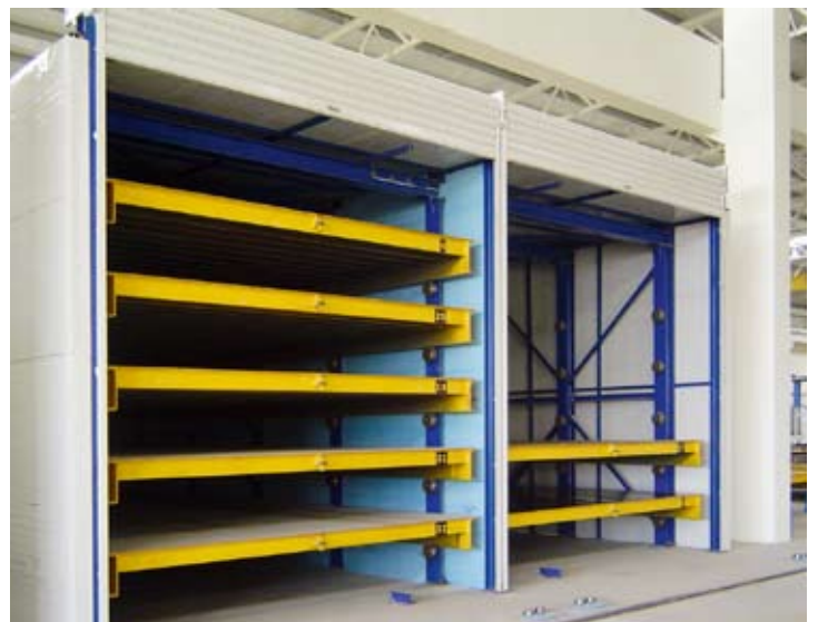
First-In, First-Out Curing System with roller- shutter doors on the entry and exit openings.
