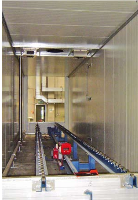
First-In, First-Out Curing System with roller- shutter doors on the entry and exit openings.
